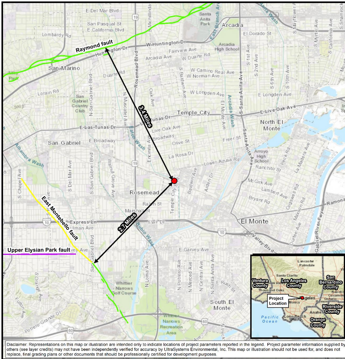
Figure 4.7-2 REGIONALLY ACTIVE FAULTS
