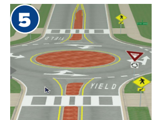
Low Cost Traffic Calming Circle
