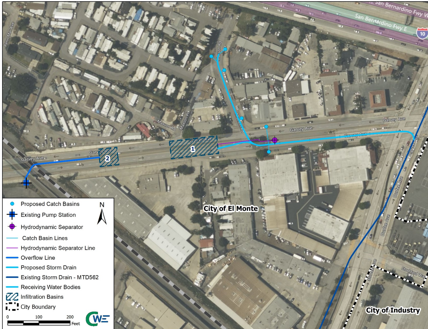
Figure 2-2 Proposed Storm Drain Alignment and Infiltration Gallery
