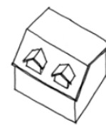
Roof with Dormer Windows
